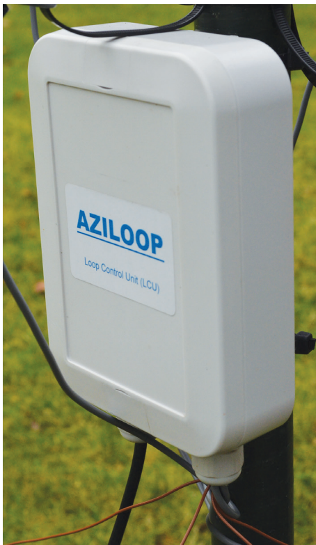
FIGURE 2: The DF-72 loop control unit (LCU).
